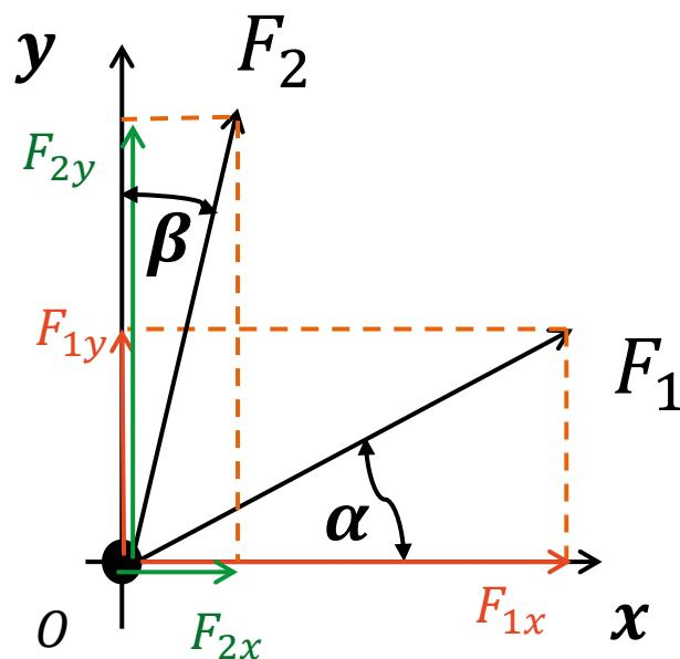
$$\begin{array}{ll} F_{1x} = F_1 * \cos\alpha & F_{2x} = F_2 * \sin\beta \\ F_{1y} = F_1 * \sin\alpha & F_{2y} = F_2 * \cos\beta \\ \hline X_R = \sum_{i=1}^n X_i = F_{1x} + F_{2x} & F_R = \sqrt{X_R^2 + Y_R^2} \\ Y_R = \sum_{i=1}^n Y_i = F_{1y} + F_{2y} & \tan\alpha_R = \frac{Y_R}{X_R} \end{array}$$
