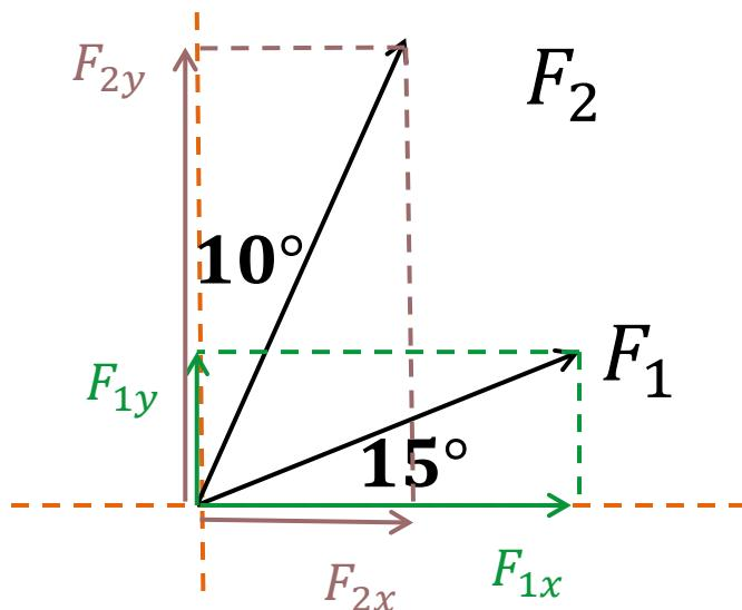
$$X_R = \sum_{i=1}^n X_i = F_{1x} + F_{2x} \quad Y_R = \sum_{i=1}^n Y_i = F_{1y} + F_{2y}$$
